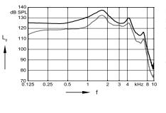
Max. Output sound pressure level (L = 90 dB)
