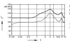
Max. Output sound pressure level (L = 90 dB)
