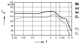
Max. Output sound pressure level  $(L_1 = 90 \text{ dB})$
